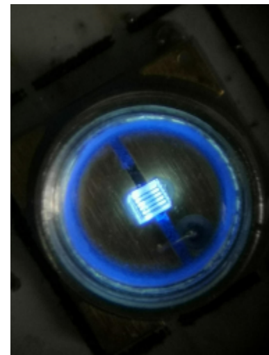
“Devil's Eye” : UVC chip in center Blue phosphor around
